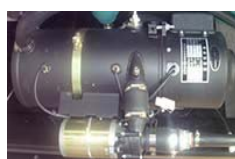
Diesel powered heater
